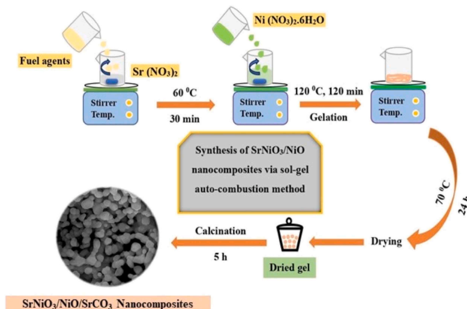
Fig. 1. : Schematic of the synthesis of SrNiO 3 /NiO/SrCO 3 nanocomposites.
